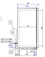
Drain Electrical inlet (power) RΩ Refrigerant Outlet
